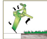
The rod rearms automatically with the simple lifting of the implement.
