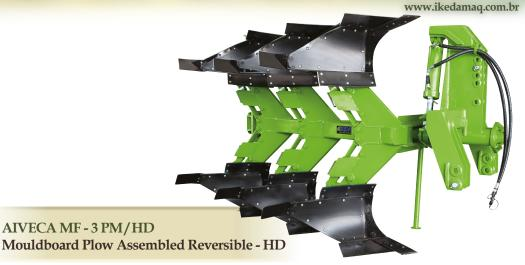
The Mouldboard Plow Assembled Reversible, of HD line is indicated for extra heavy work where plowing in both directions produce significant yield gains. Its reversion is done through the cylinder triggered by the tractor hydraulic system.
